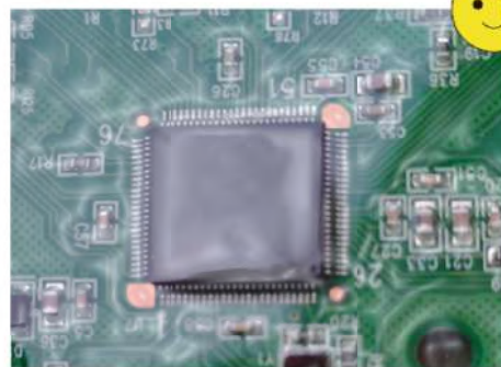
After coating with three anticorrosion layers
