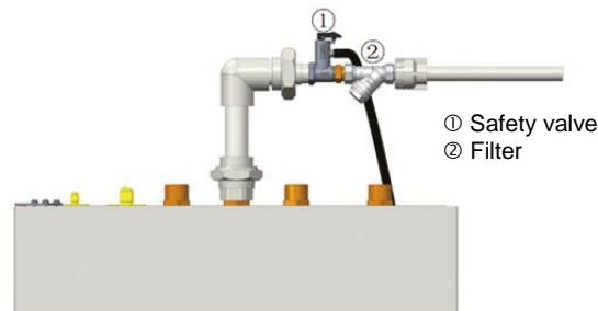
Installation mode 1: Safety valve on the water supply from the water network (inlet water pressure = 0.1–0.5 MPa)
