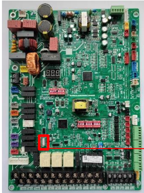
Main control PCB
